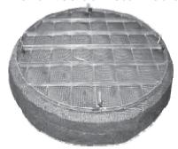
The demister pad/mist eliminator is made by Monel 400, Monel 400 is a nickel-copper alloy (about 67% Ni – 23% Cu) that is resistant to sea water and steam at high temperatures as well as to salt and caustic solutions. and it is constructed from multi layer knitted mesh media and provides a dense 'mat' through which process gas flows and liquid entrainment is trapped through coalescence and prevented from passing downstream, achieving liquid/gas separation.
